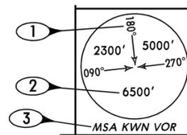
NOTE: Normal coverage is a 25 NM radius from the forming facility/fix. If the protected coverage is other than 25 NM, that radius is depicted below the forming facility/fix.
