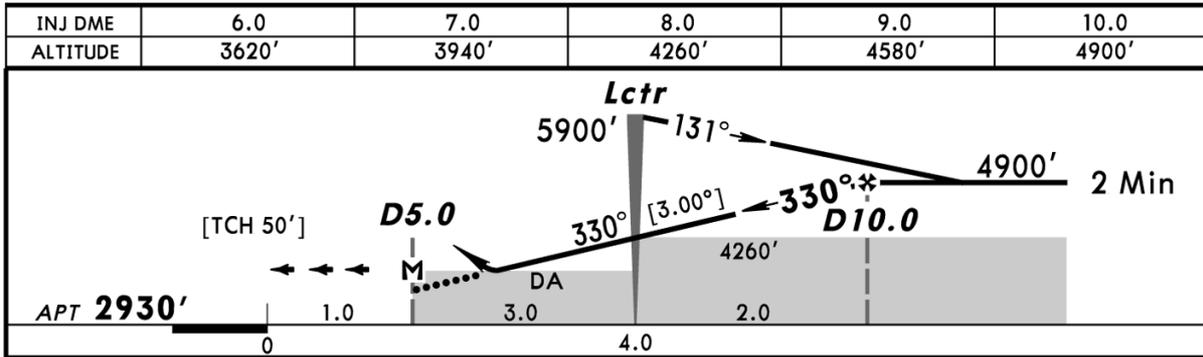
In exceptional cases it may be necessary to include CDFA and non-CDFA minimums. Where this occurs, a level segment is shown prior to the missed approach point and the pull-up arrow is shown at the MAP.
