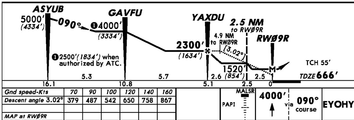
The descent angle accuracy may be affected by temperature. When the outside air temperature is lower than standard, the actual descent angle will be lower. Check your avionics equipment manuals since some compensate for nonstandard temperatures.
